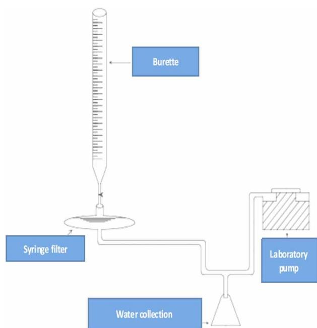
**Figure 1** | The design of the biofilter used in the experiment.
